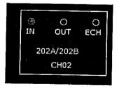
When the Manual point operation is over, after putting the KEY in the KLCR, A KEY OUT flashing indication will appear on the VDU, Now the SM/ ASM has to Lock the control for the Steady indication. A Crank handle locked Green indication will appear when the particular Crank Handle has locked by SM /ASM by clicking the RECEIVE CONTROL menu.
