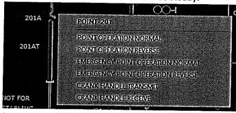
3. After inserting CH KEY to CH EKT Box CH KEY OUT indication will flash. SM should receive CH KEY by using RECEIVE CONTROL menu in concerned crank handle button. After that IN steady Indication will display.
